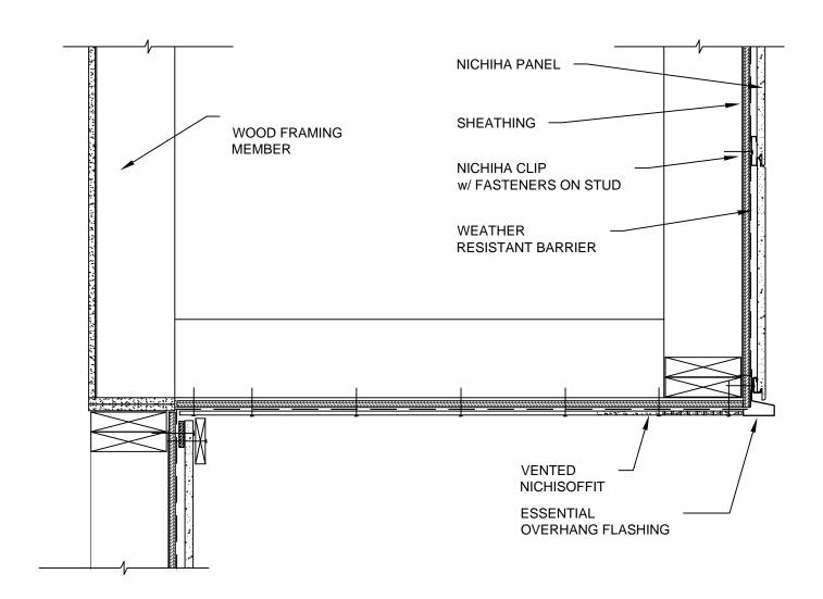
10MM - WOOD STANDARD 6' & 10' HORIZONTAL PANEL & NICHISOFFIT DETAIL
