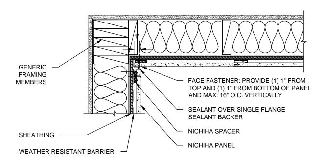
10 MM - SHEATHING METHOD - 10' VERTICAL PANEL INSIDE CORNER DETAIL
