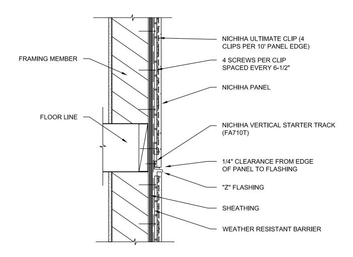
10MM - STANDARD - 10' VERTICAL PANEL COMPRESSION JOINT DETAIL
