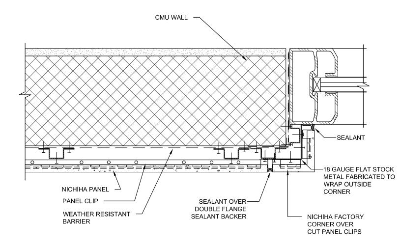
10 mm - CMU - RECESSED WINDOW JAMB DETAIL WITH FACTORY CORNER
